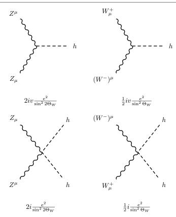
The interaction between one scalar and two-vector bosons is always proportional to a VEV and can exist only after gauge symmetry breaking.
