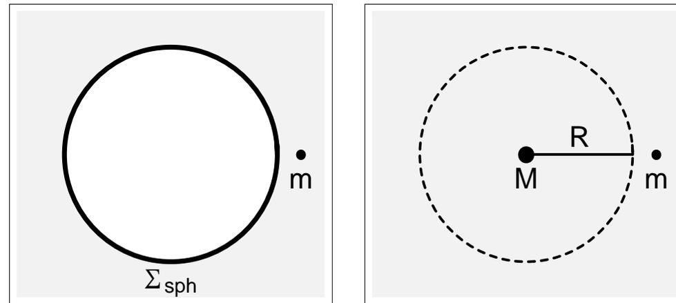
Left panel: Spherical holographic screen  $\Sigma_{\text{sph}}$  with area  $A = 4\pi R^2$  and test mass  $m$ . Space has emerged outside the screen  $\Sigma_{\text{sph}}$ , which has  $N$  microscopic degrees of freedom at an equilibrium temperature  $T$  with total equipartition energy  $E = \frac{1}{2} N k_B T$ .
